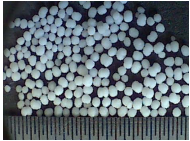
Figure 19 Dried pellets obtained from the spheronisation of 55 wt.% water-MCC extruded at V = 690 \text{ mm s}^{-1} through a 1 mm diameter die with L/D = 2 .
